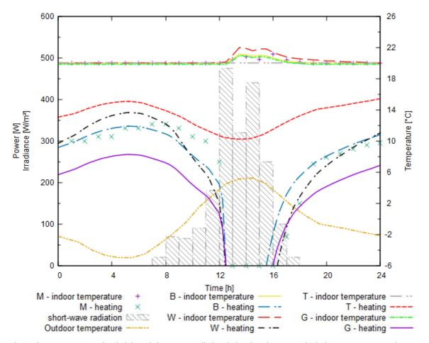
Figure 2: Outdoor temperature at 2 m height and short-wave radiation during the winter scenario, indoor temperatures and power needed for heating in room S for different building scenarios (Basic, big Windows, Trees, Green roof and facades)
