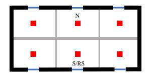
Figure 1: Floor plan of the simulated building. With window positions as small blue lines, heating grid points as red squares, centered north room on 2nd floor N, centered south room on 2nd floor and reference to measurements S, centered south room on 3rd floor under the roof RS.
