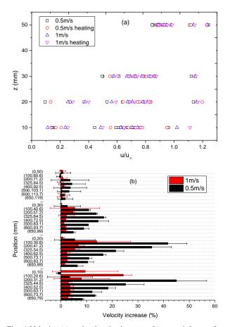
Fig. 4 Velocity (a) and velocity increase (b) at each layer after heating the rooftop
