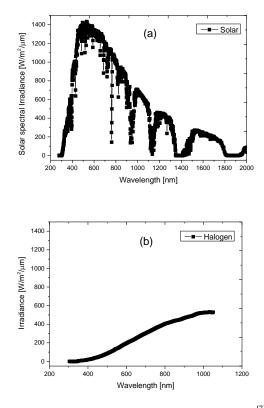
Fig. 3 Comparison of irradiance between (a)  $\operatorname{solar}^{[7]}$  and (b) halogen radiation
