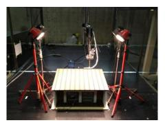
Fig. 2 Configuration of halogen lamps
