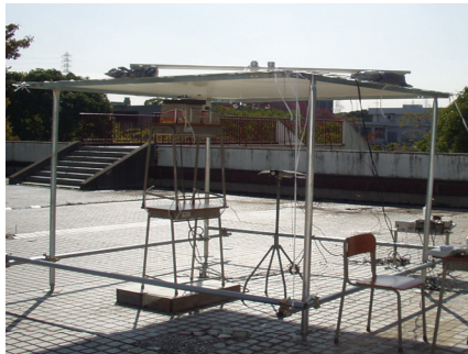
Figure 2 Field measurement of solar reflectance and transmittance for membrane material
